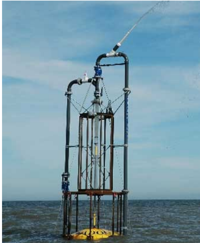
Figure 33 SeaDog Prototype Deployed of Galveston Texas (note the water jet discharge from the top)
