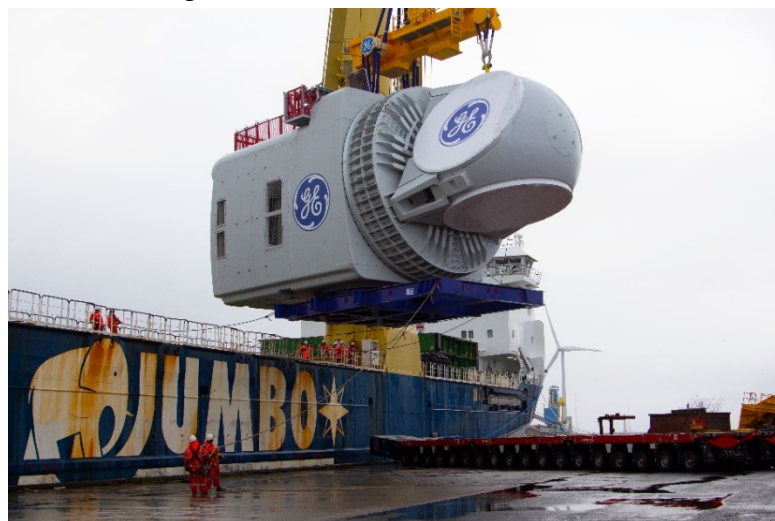
Figure 15 GE 12.5 MW Direct Drive Nacelle (Source: GE Renewables)
