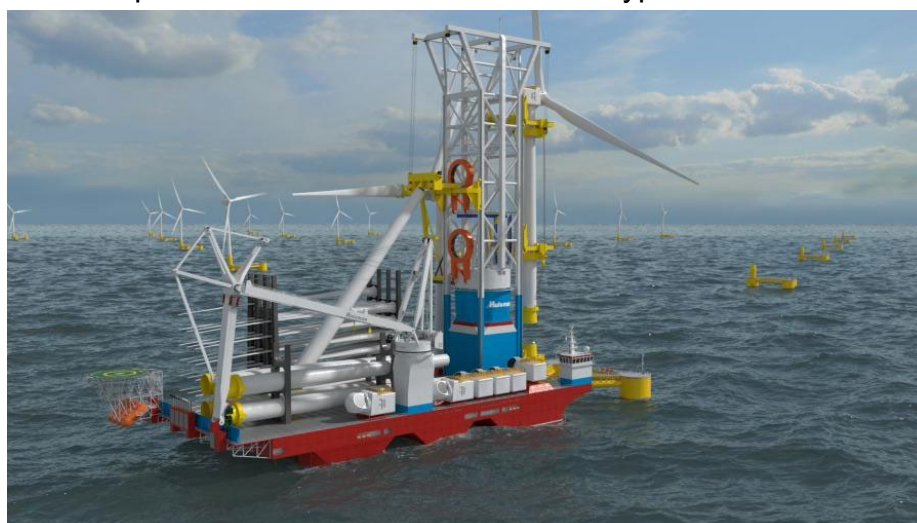
Figure 25 3D Rendering of Huisman Windfarm Installation Vessel
