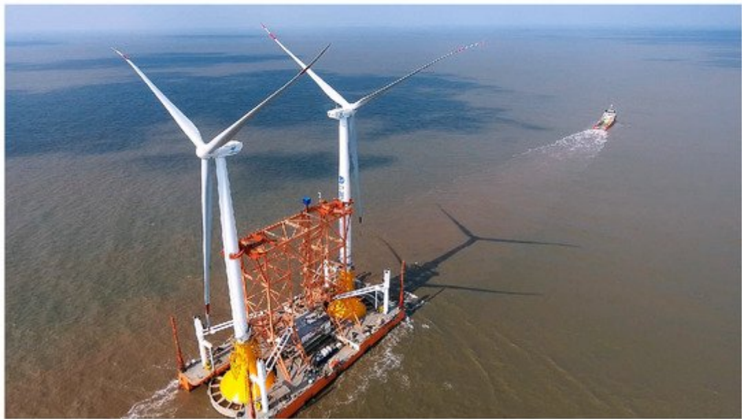
Figure 21 the Tianjin University and Daoda Company Composite Bucket Foundation (CBF)
